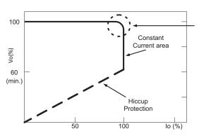
Typical LED power supply I-V curve
